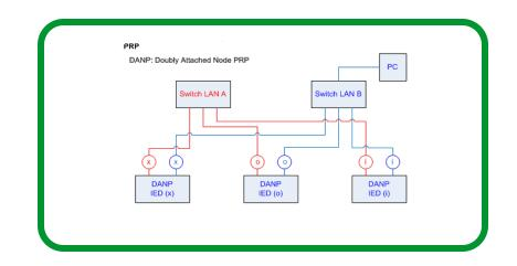
If for any reason an IED fails, only its protection function is lost. The other IEDs continue to communicate over the redundant LAN to protect and control electrical equipment.
