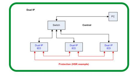
In this scheme, communication to the control system is over a standard single communication network, and the protection scheme to the local IEDs uses the HSR protocol in order to avoid additional switching and to increase the communication availability. (A single network could be used but is not recommended, and the PRP protocol is also possible but costs more.)
