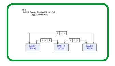
If for any reason an IED fails, its protection function and the communication redundancy are lost, but the other IEDs continue to communicate, protect, and control the electrical equipment through a single communication network.
