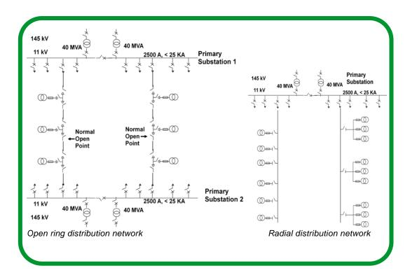
Open rings are often used to increase the availability of power. A first level of improvement consists of connecting the two ends of the ring to two possibly different primary substations. This architecture offers redundant supply for each ring, with a smaller proportion of the load disconnected in case of a primary substation blackout.
